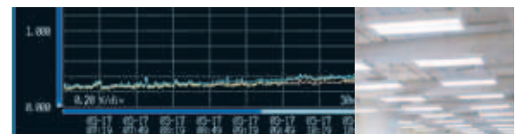
The PQ3100 can simultaneously record 3 channels of ΔV10 and IEC flicker data.
